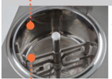
It is a real "technological pot" with a very large bottom surface area thanks to the ratio between diameter and depth. Thermal exchange is optimized without burning or sticking any product inside, even if very delicate or in small quantity.
