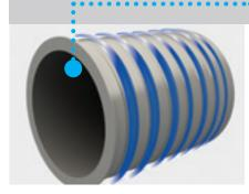
Refrigerant gas direct expansion system on the batch freezing hollowed spiral cylinder having a progressively variable diameter to optimize the chilling performance on the whole cylinder surface.
