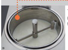
The stirrer plays an important role in the heating process. It is provided with a patented counter-stirrer, easily and completely dismountable. It guarantees a fast dispersion and solubilization of solid ingredients into liquid ones.
