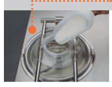
Double lid with opening system actuated by servo-assisted hydraulic pistons for easy ingredient introduction even in case of product in progress. The machine has not to be stopped in full compliance with certified EC safety regulations.
